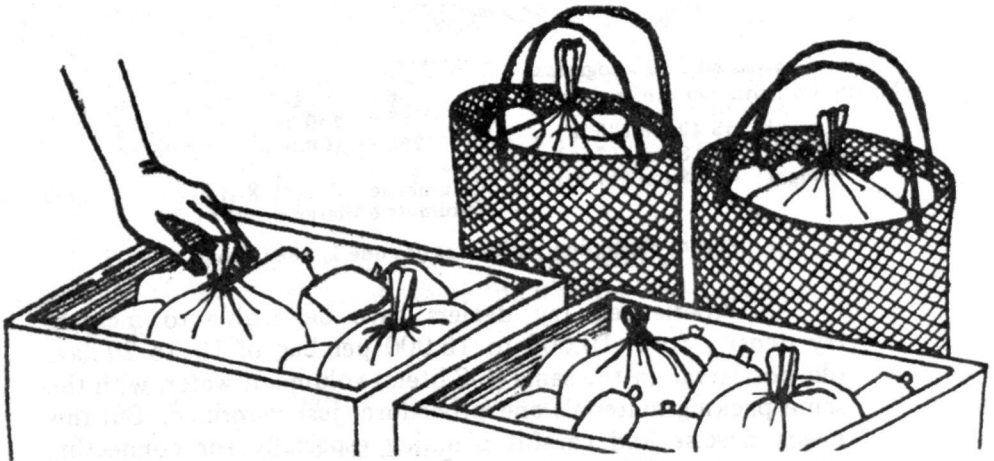
Fig. 12. Pack plastic bags in styrofoam boxes with ice to maintain the low temperature of transport water.
