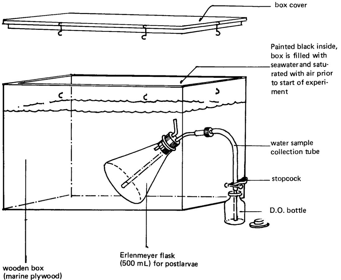
Dissolved oxygen concentrations were determined using the Winkler method (5) on 100 mL samples drawn from the respiration chamber. Water was allowed to flow through the chamber (about 500 mL) to replace the water inside the chamber with that saturated with air before drawing the sample for initial dissolved oxygen readings. Water was again drawn after allowing the animals to respire for a specified length of time.
