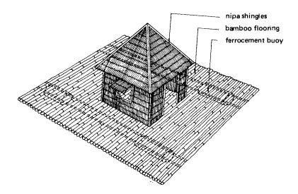
The buoys may be used in the construction of a raft house. The raft house serves as guardhouse and storage for feeds and other equipment used in the culture of mussels, Fig. 3 shows a typical arrangement of a raft house made of bamboo.
