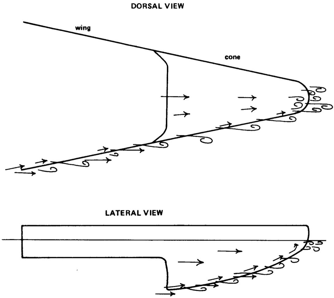
Figure 2. Probable stream-line in operating the fry sweeper.
