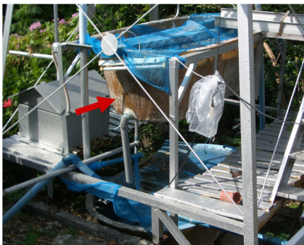
Fig. 20. Physical filtration. The tank (red arrow) is packed with sand, gravel and charcoal. Water is filtered and pumped to an overhead reservoir before recirculating to the rearing tanks.
