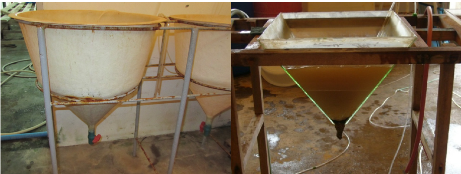
Fig. 33. Sample of conical incubation jars for Artemia , made of fiberglass (left) and glass (right).
