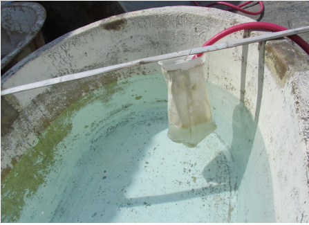
Fig. 17. Seawater is filtered prior to use in the hatchery.
