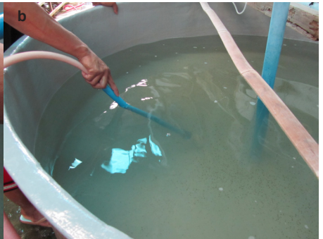
Fig. 29. Leading end of siphon may be fitted with a brush (a) to scrub the tanks during cleaning (b).
