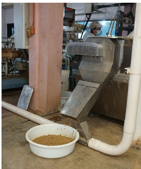
The new extruder at SEAFDEC/AQD's feed mill used to produce aquaculture feeds. Photo by RH Ledesma
