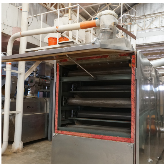
The new 5-layer dryer replaces the ovens previously used to dry feeds. Photo by RH Ledesma
