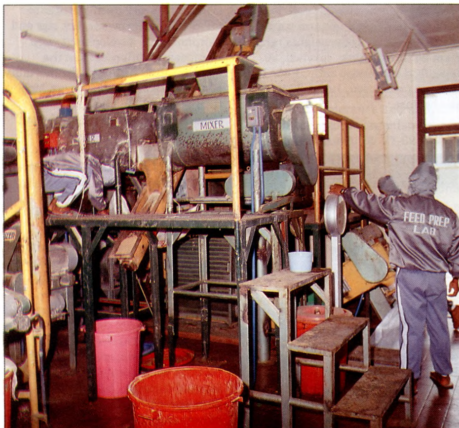
The pilot feed mill at AQD can produce 50 tons of feed a day for experiments and maintenance of fish stocks.
