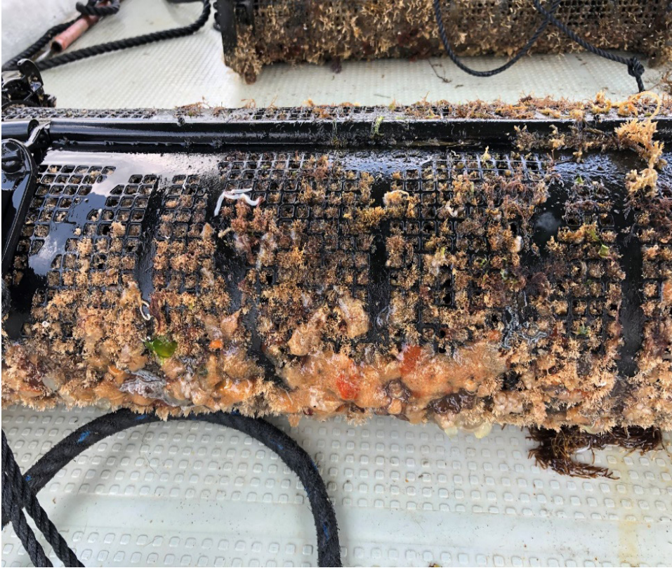
Figure 4. Intensive biofouling on an oyster culture basket hung from a red seabream culture cage.
