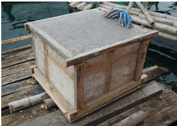
Figure 15. Concrete block as mooring/anchor device to stabilize the position of the cage
