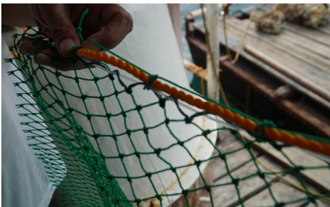
Figure 8. Attachment of polynet #14 to PE rope #10 using a nylon line as a guide
