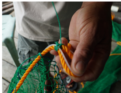
Figure 9. Fabrication of an eyelet in every corner of the net as a provision for attachment to the framework
