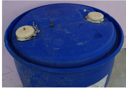
Figure 14. Plastic drums with tire valves for filling in of compressed air
