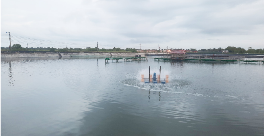
Figure 6. Provision of paddle wheel in the course of low dissolved oxygen in the pond
