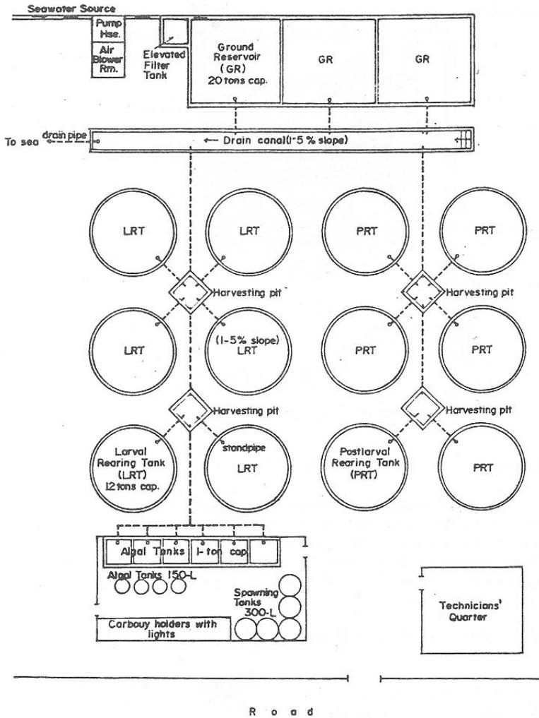
Fig. 11. A sample layout of a prawn hatchery.
