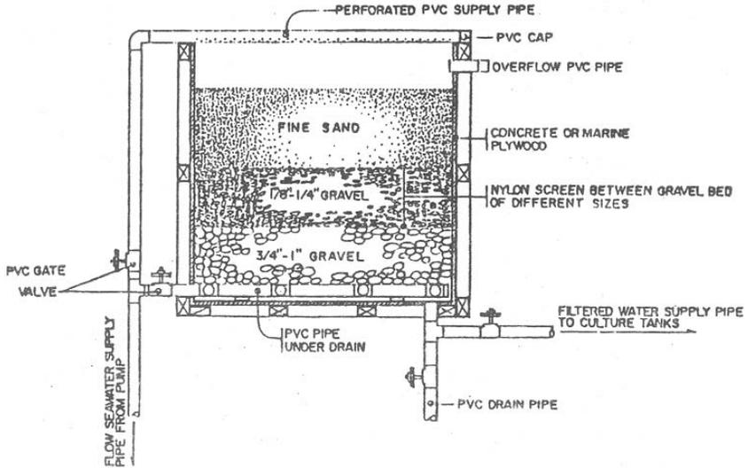
Fig. 10. Cross-section of a sand and gravel filtration unit.
