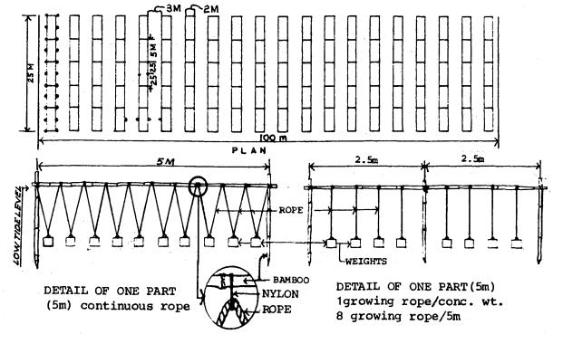
Figure 4. Fixed structure mussel farm using bamboo plots.
