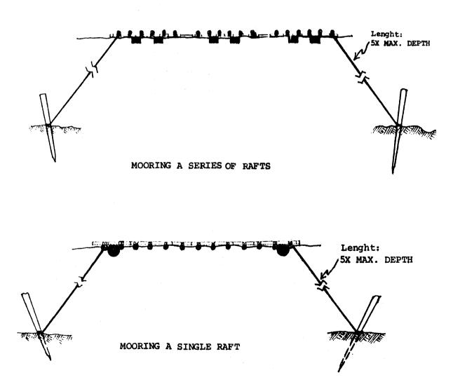
Figure 5. Methods of mooring a single raft or a series of rafts,
