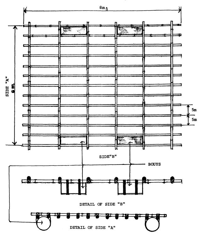
Figure 2. Construction detail of a mussel raft using bamboo framework and floats.
