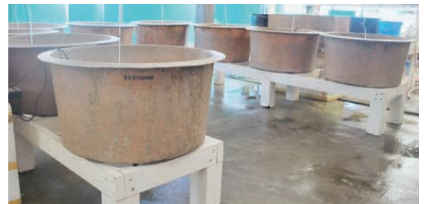
[TOP] Recirculating tank system used for looking at the effects of higher water temperatures (29-33°C) on the reproductive performance of rabbitfish. Note the water heater (small orange box) and its thermostat (big orange boxes). [ABOVE] Set-up for the larval rearing experiments where the water is maintained by small heaters with thermostat. This set-up is used for milkfish, seabass and rabbitfish
