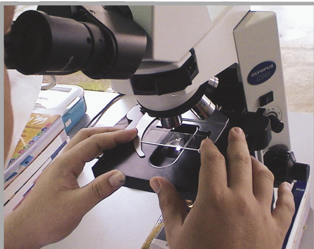
6 Place the slide on the microscope stage and adjust focus starting with the lowest power objectives before switching to higher magnifications
