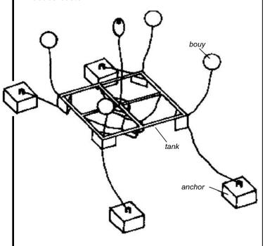
The design measures 10×10×1 m, and can be installed at 30 m depth. It can withstand 3-m waves coming every 8.5 sec and strong currents. - MTC
