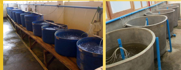
Polyethylene (left) and fiberglass (right) larval rearing tanks. Larval rearing tanks can range from 100 L capacity to several tons, depending on capacity and target production.
