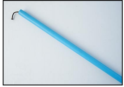
Fig. 13. PVC pipe with hook for pulling boxes
