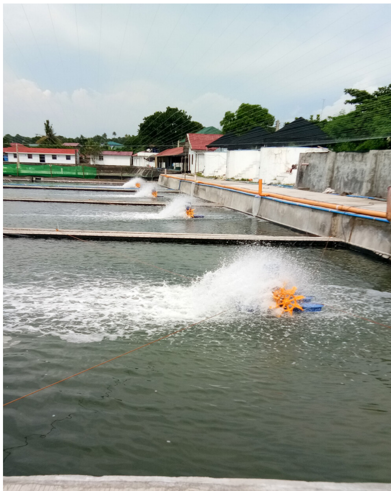
Use of paddle wheel aerators as life support system for the shrimps in Butong, Taal, Batangas. Photo by R Traviña
