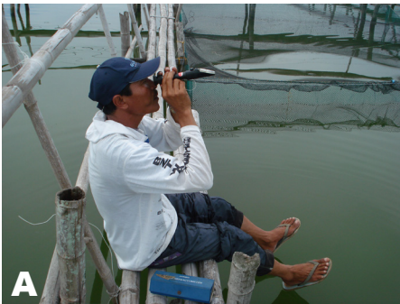
Figure 21. Instruments used in monitoring water parameters: refractometer for salinity (A), D.O. meter for dissolved oxygen and temperature (B), and pH meter for pH level (C)
