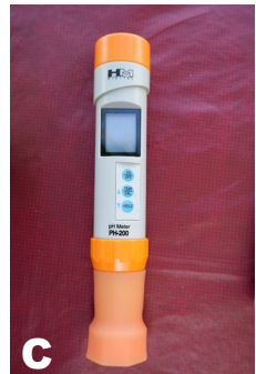
Figure 21. Instruments used in monitoring water parameters: refractometer for salinity (A), D.O. meter for dissolved oxygen and temperature (B), and pH meter for pH level (C)
