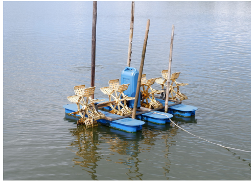
Figure 22. Electric-powered paddlewheel (1 hp)
