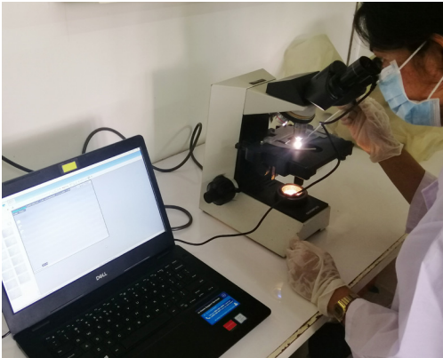
Figure 13. Capillary pipette technique. Mixed sample of microalgae is observed under the microscope and a Pasteur pipette with very fine tip is used to pick up cells of desired microalgae
