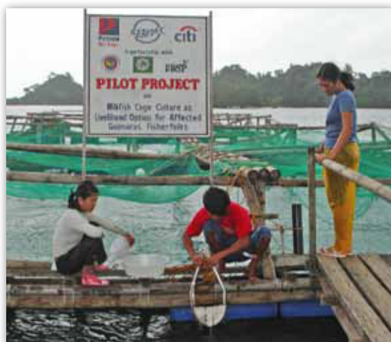
Monitoring sediment quality in Igang Mariculture Park using a fabricated Ekman grab
