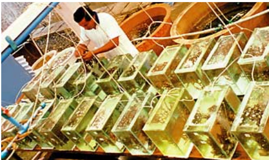
Experimental set-up for the study on sequestration of heavy metals by the thalli and agar of seaweed
